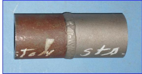
Figure 1. Metallurgical tube sample section representing dissimilar metal weld joint of stainless steel material to lower-alloy steel material. As can be seen above, it is at this type of weld location that any failures occur as a result of the temperature induced stress, carbon diffusion and oxidation resistance.]
