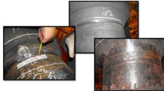
Figure 4. Images of the indication which required weld repair.
