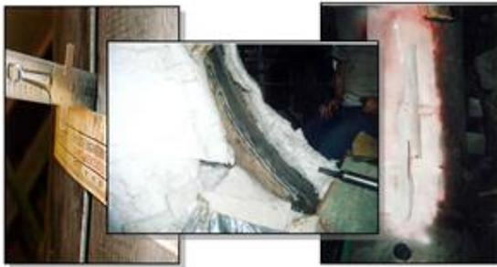
Figure 6. Images of the through-wall crack which required weld repair.
